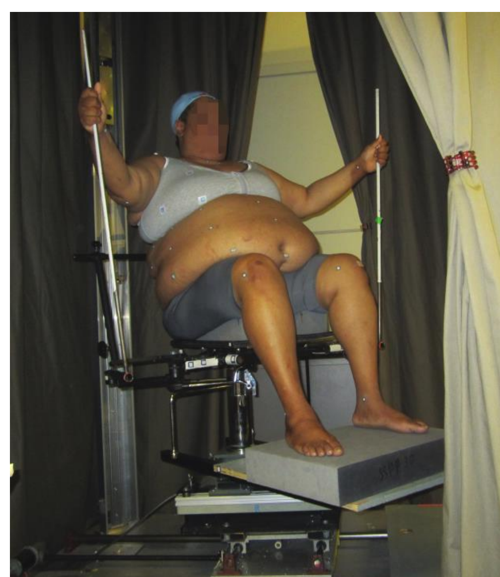
Adjustable seating fixture to replicate relevant postures
